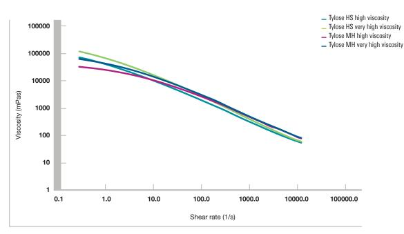
measured at 20 °C, water 20 °dH (German hardness), 1.9 % solutions
