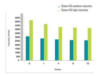
Testing of Tylose MH and HS solutions ( Brookfield RV at 20  $^{\circ}$ C, 1 %) at different exposure times up to 12 weeks at pH 6.5 and pH 9.8
